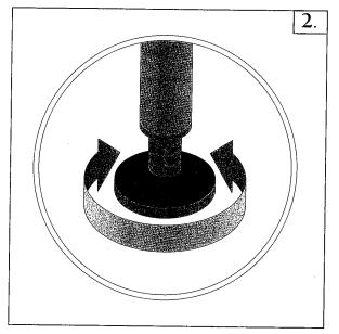
Adjust the height of each leg in  $1\ \mathrm{cm}$  increments. Otherwise, there is a danger of twisting the table frame.
