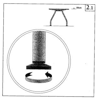
Turning the adjusting screw to the right lowers the top of the table to a minimum height of 68 cm.
