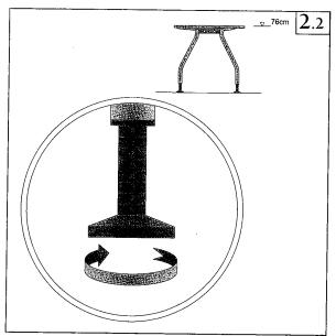
Turning the adjusting screw to the left raises the top of the table to a maximum height of 76 cm.
