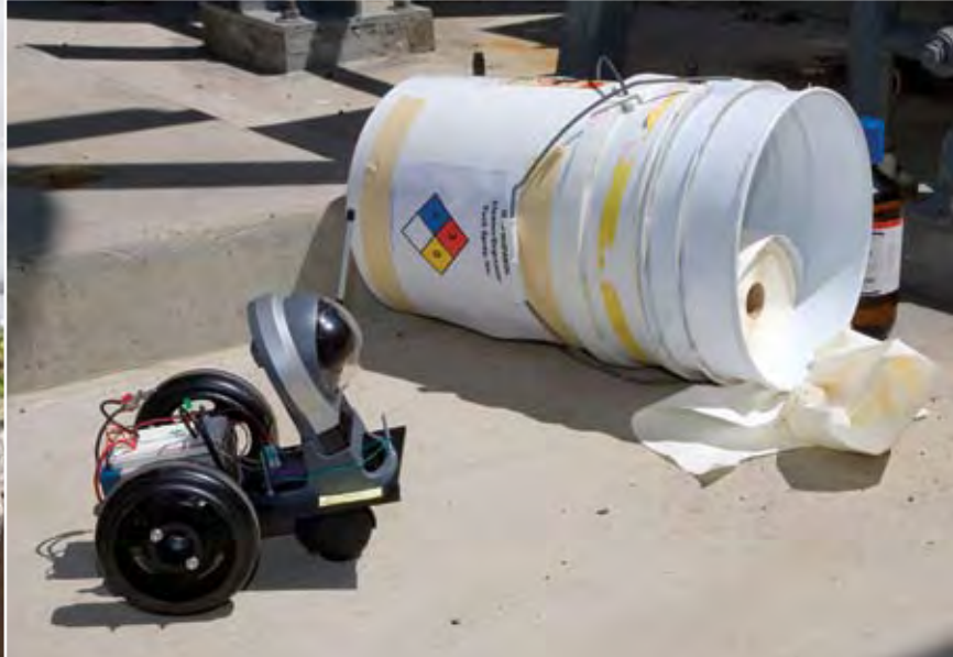
At left and above: At a recent emergency drill, ResCUE team members Naveen Ashish (left) and Anton Popov track images sent by the autonomous mobile sensing platform, which “reads” the label on a mock spilled chemical container. At right: Chris Davison guides the sensing platform while watching its progress in his goggles.
