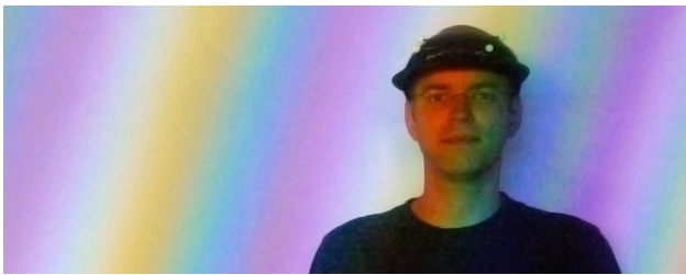
Figure 4: The repeating channel array, with solid colors projected onto a user and a white card at the plane of focus.
